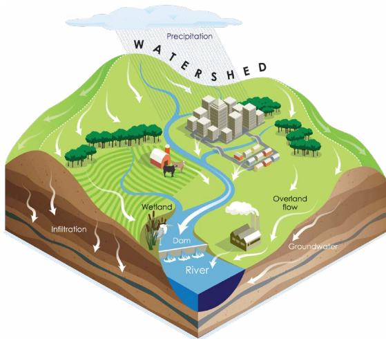
Figure D3 ■ Precipitation absorbed by the watershed, through specific catchment areas
